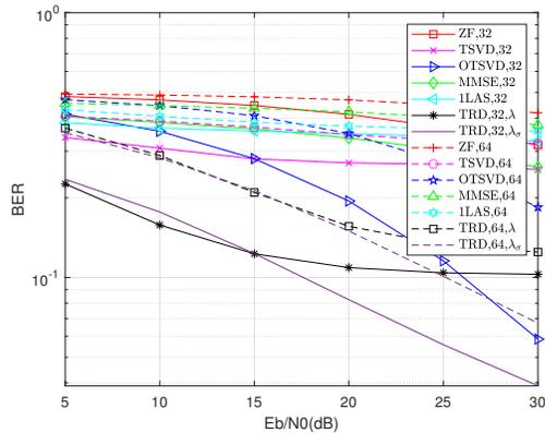
Fig. 4. BER versus SNR for the  $512 \times 64$  and  $512 \times 32$  XL-MIMO.
