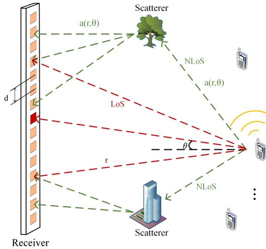
Fig. 1. The mixed LoS/NLoS near-field channel model for XL-MIMO.
