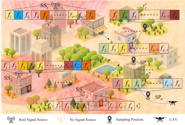
Fig. 2. 3D compressed wideband spectrum mapping model. SS_j represents the j -th signal source (there may be a real signal source or no signal source) of all n positions, the UAV equipped with a spectrum monitoring device flies to m out of n positions to sense p out of q frequency points at each position.
