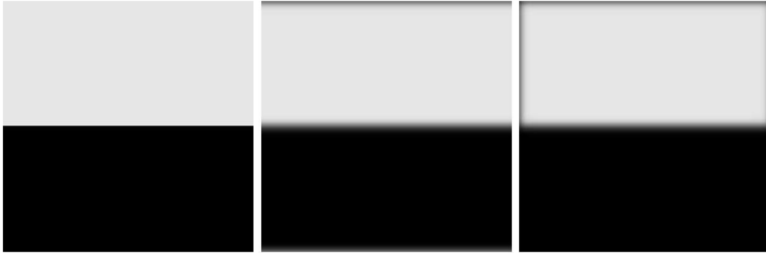
FIGURE 4.32 (a) A simple image. (b) Result of blurring with a Gaussian lowpass filter without padding. (c) Result of lowpass filtering with padding. Compare the light area of the vertical edges in (b) and (c).
