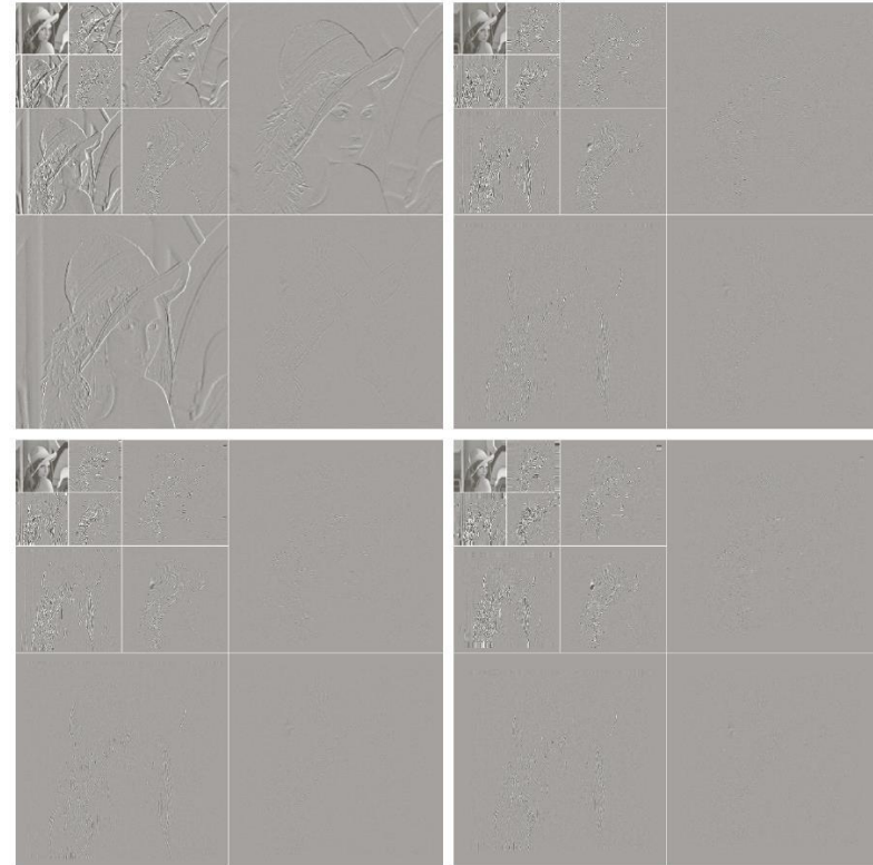
FIGURE 8.46 Three-scale wavelet transforms of Fig. 8.9(a) with respect to (a) Haar wavelets, (b) Daubechies wavelets, (c) symlets, and (d) Cohen-Daubechies Feauveau biorthogonal wavelets.
