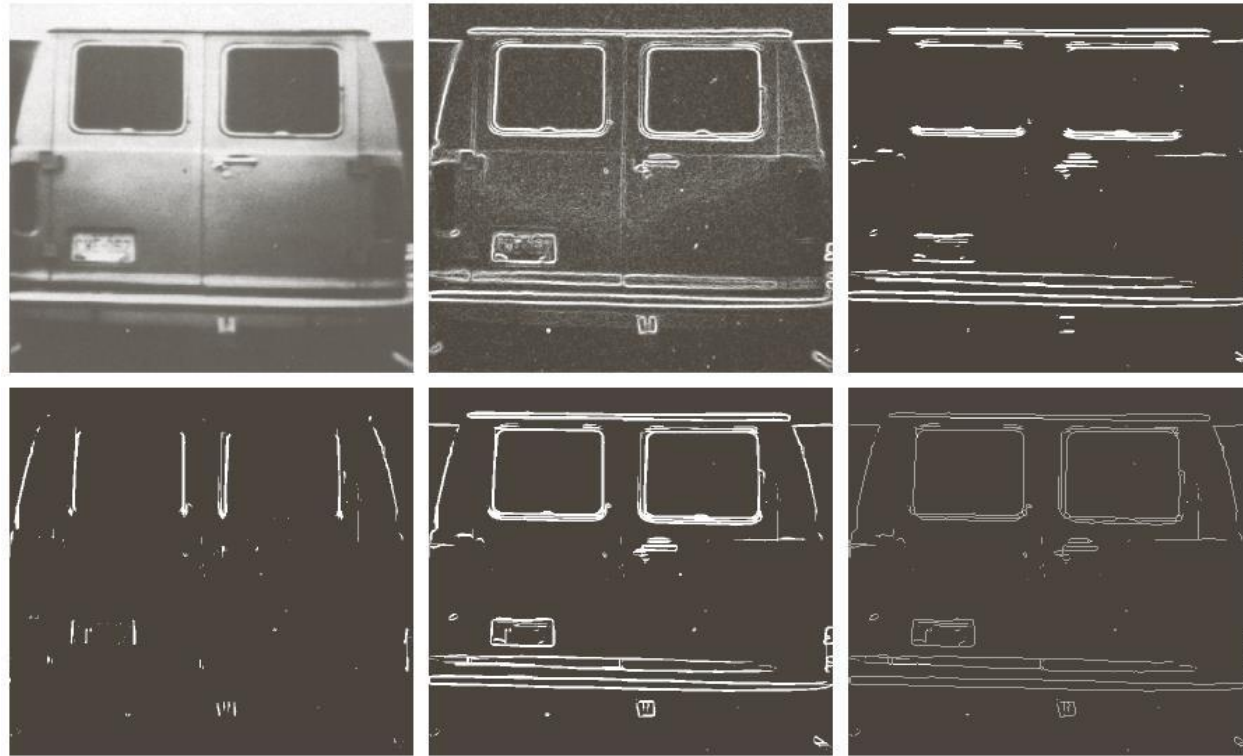
FIGURE 10.27 (a) A 534 \times 566 image of the rear of a vehicle. (b) Gradient magnitude image. (c) Horizontally connected edge pixels. (d) Vertically connected edge pixels. (e) The logical OR of the two preceding images. (f) Final result obtained using morphological thinning. (Original image courtesy of Perceptics Corporation.)
