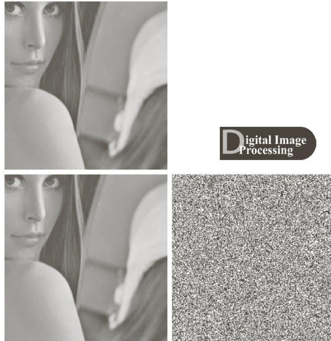
FIGURE 8.51 A simple invisible watermark: (a) watermarked image; (b) the extracted watermark; (c) the watermarked image after high quality JPEG compression and decompression; and (d) the extracted watermark from (c).
