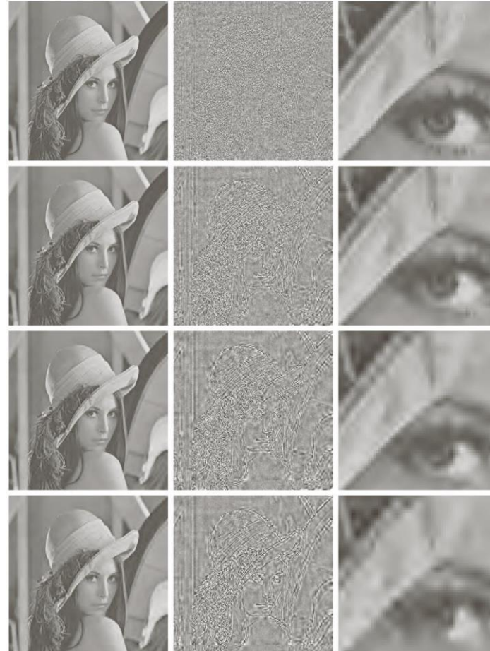
FIGURE 8.49 Four JPEG-2000 approximations of Fig. 8.9(a). Each row contains a result after compression and reconstruction, the scaled difference between the result and the original image, and a zoomed portion of the reconstructed image. (Compare the results in rows 1 and 2 with the JPEG results in Fig. 8.32.)
